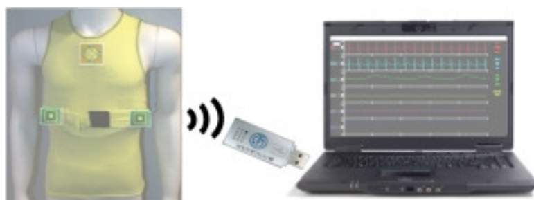
Depiction of the wearable 3-lead IMAGE sensing device attached to the sleeveless exercise shirt (picture courtesy of CSEM SA, Switzerland)
